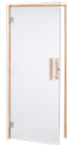
DS80 sauna door, clear class 3-sided frame, 8 mm single pane safety glass, hinges can be attached on left or right Glass: 824 x 1997 mm Spruce frame: 920 x 2060 x 80 mm Item no. DS80-3CS-824 (824 mm)
